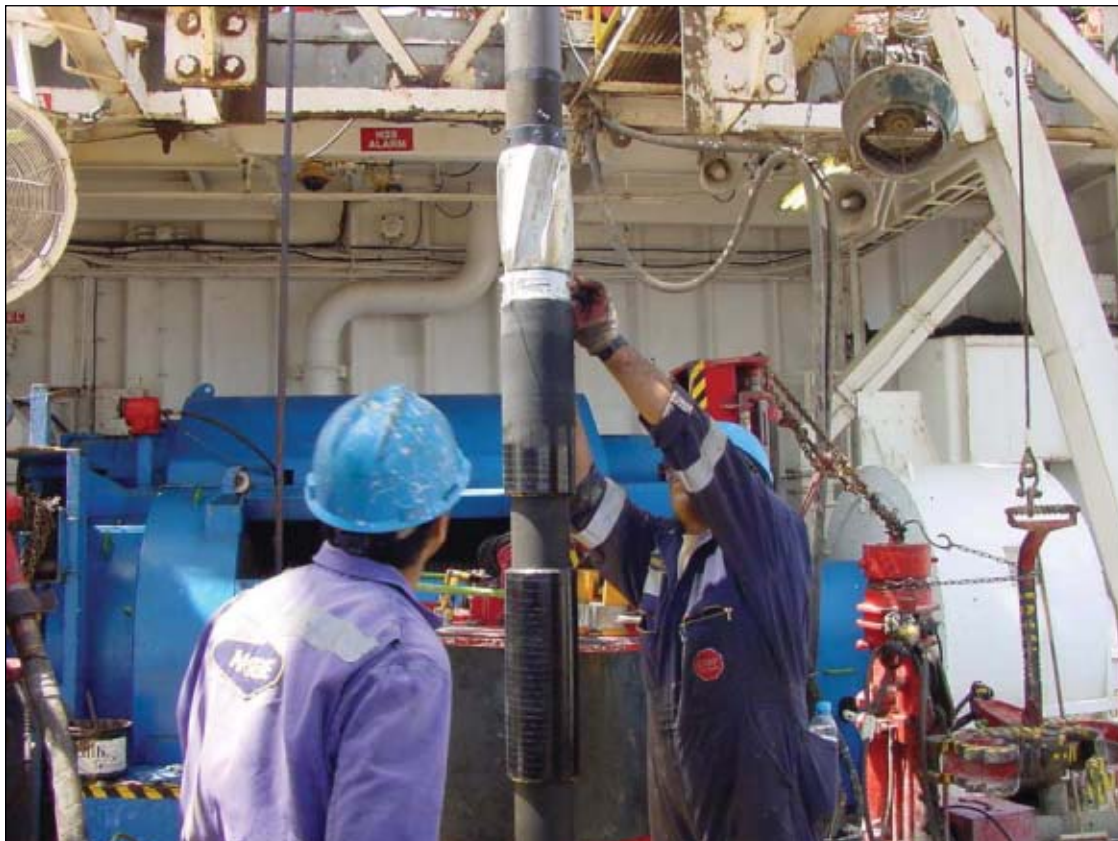
Dubai Petroleum Exploration runs a water-swelling E-ZIP external packer in Rashid field, off Dubai. DPE ran 25 of these packers in the Fateh, SW Fateh, and Rashid fields, April-May 2006. Photo from Swellfix.
